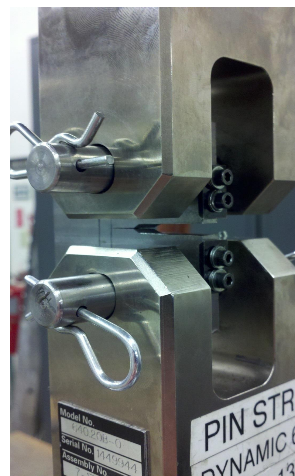
Figure 2: K_{IC} testing setup
